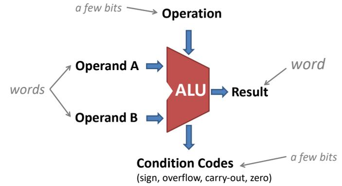
Hardware unit for arithmetic and bitwise operations.
