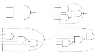
Multi-input OR gates with can be created analogously. Multi-input NAND and NOR gates can be created by inverting the outputs of multi-input AND and OR gates.
