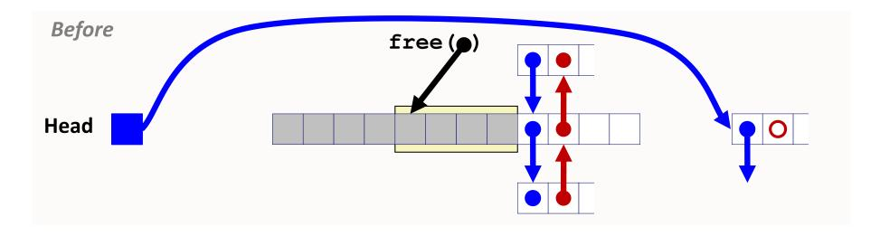
Splice out successor block, coalesce both memory blocks and insert the new block at the head of the free list.
