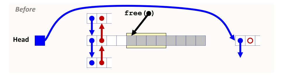
Splice out predecessor block, coalesce both memory blocks, and insert the new block at the head of the free list.
