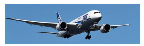
"... a Model 787 airplane ... can lose all alternating current (AC) electrical power ... caused by a **software counter** internal to the GCUs that will overflow after 248 days of continuous power. We are issuing this AD to prevent loss of all AC electrical power, which could result in loss of control of the airplane." --FAA, April 2015
