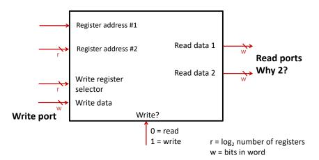
Array of registers, with register selectors, write/read control, input port for writing data, output ports for reading data.
