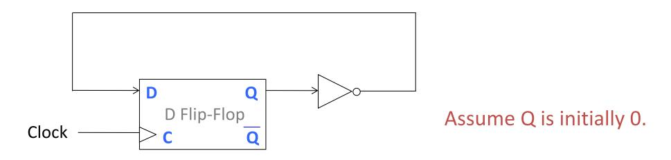
Moral: It's OK to use the current output Q of a flip-flop as part of the the next data input D to the same flip-flop.
