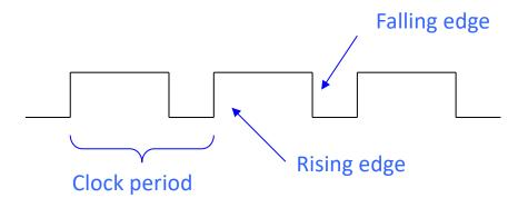
A clock controls when to update a sequential logic element's state.
