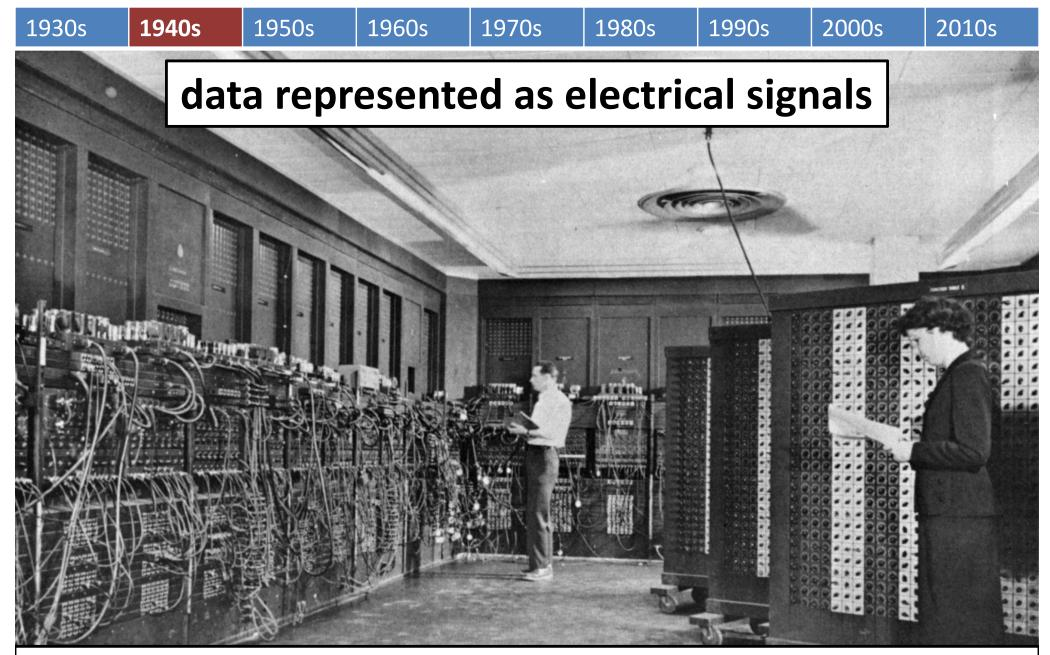
**ENIAC** (Electronic Numerical Integrator and Computer), First Turing-complete all-electronic programmable digital computer. University of Pennsylvania, 1940s
