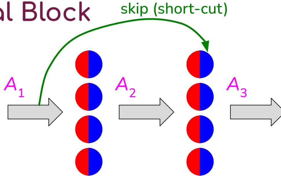
$A_1 \xrightarrow{\text{Linear}} Z_2 \xrightarrow{\text{Activation}} A_2 \quad A_2 \xrightarrow{\text{Linear}} Z_3 \xrightarrow{\text{Activation}} A_3$
