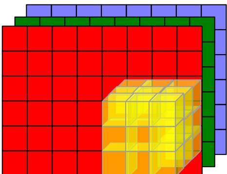
$$\begin{matrix} * & \begin{matrix} \text{Input Volume} \\ \text{Kernel} \end{matrix} & = & \begin{matrix} \text{Output Volume} \end{matrix} \end{matrix}$$
