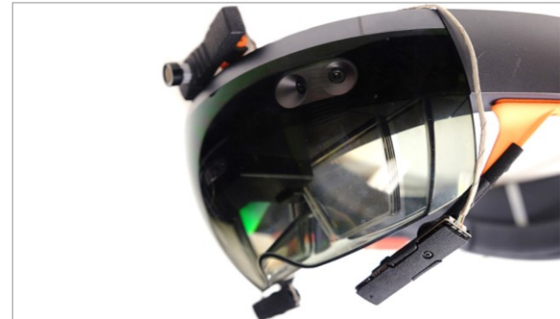
Figure 1. The Microsoft HoloLens with an attached Pupil Labs high speed binocular eye-tracker.
