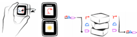
Figure 2 , Eugenie++ provides gestural and tangible interaction techniques for browsing large data sets: (left) tilting to search, neighboring for traversing an hierarchical database; (right) stacking to collapse and expand biological constructs.
