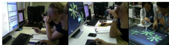
Figure 3, Comparing similarity search results on the three experimental conditions: traditional GUI with multiple Firefox windows displaying UCSC Gnome Browser, JAX Mice, Entrez Gene and NCBI Blast (left); a multi-mouse implementation of G-nome Surfer 2.0 running on the Microsoft Surface (center), physical interaction objects were replaced with buttons; G-nome Surfer 2.0 (right).
