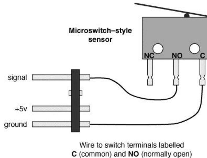
Perhaps the most commonly used of all robotic sensors, the “touch sensor” is nothing more than a simple electrical switch; when the lever is pressed an electrical circuit is completed. Touch sensors were used in making *Sciborg*'s bumpers. *Chimera* used touch sensors in its head (to tell when it was being petted) and its tail (to tell when it was being pulled.) Touch sensors are also useful as “limit switches”, to indicate when some mechanism has reached the end of its travel.
